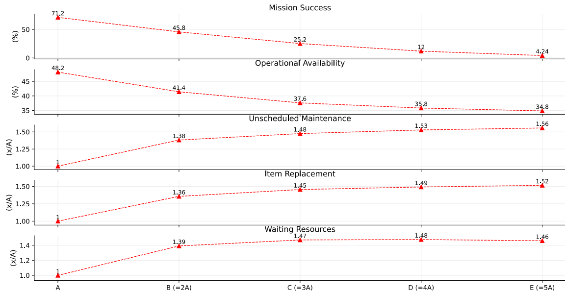
FIGURE 4.14 – Impact of Failure Rate Variation Across Multiple Performance Metrics, Including Mission Success, Availability, and Maintenance Workload.
