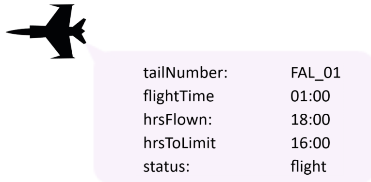
FIGURE 4.13 – Detailed Operational and Maintenance Data for an Individual Aircraft, Including Status and Flight Hours Control.
