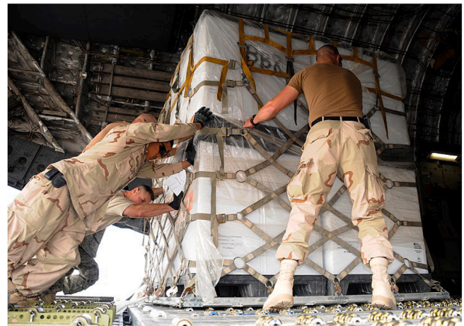
Fig. 2. A packed content on 463L pallet inside a Boeing C-17. Source: From Wikimedia Commons, the free media repository.
